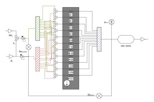
**Figure 1.** Schematic drawing of the gas diluter. Red dotted lines represent the path of  $N_2$ . Green lines represent the path of  $NO_2$ . The eleven critical orifices are placed within an aluminum block (grey). Numbers next to the orifice letters represent the flow rate relative to orifice A.
