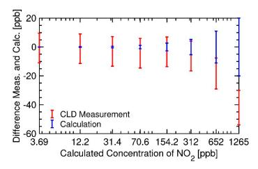
**Figure 2.** Deviation of the measured from the calculated concentrations (*x*-axis). Calculated (blue) and measured (red) values are shown with corresponding error bars and are baseline corrected to zero.
