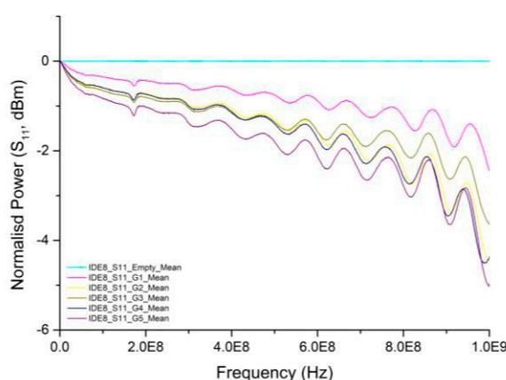
Figure 4. Spectral data between 9 kHz and 1 GHz; observation highlights a clear separation between the spectral data between 200 and 600 MHz.
