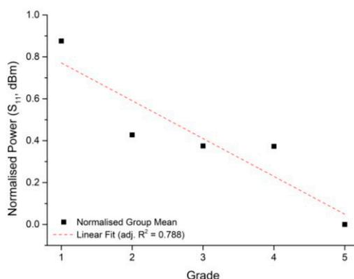
Figure 5. Correlation between strawberry grade (1–5) and sensor signal in the 200–600 MHz range.
