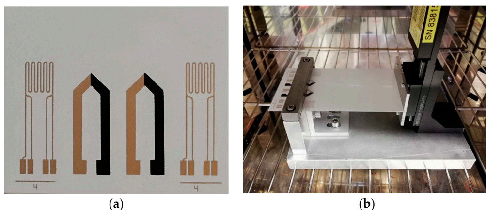
Figure 2. (a) Screen printed silver strain gauge with four wire connections and silver carbon black thermocouple printed on insulated sheet steel for bending characterization; (b) Bending test setup consisting of motorized stage and clamping.
