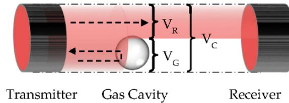
**Figure 1.** Simplified ultrasound transmission model with blocked transmission by gas cavity.
