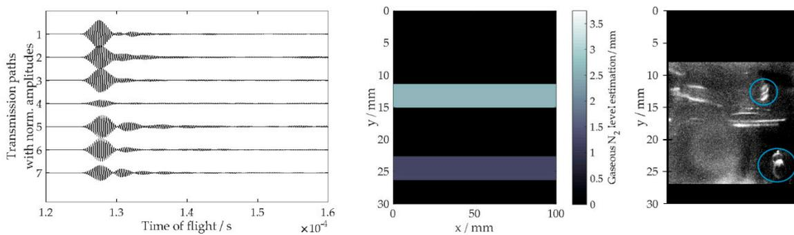
**Figure 5.** Detection of rising gaseous bubbles by ultrasound transmission measurement (received acoustic signals (left) and image plot (centre)) and recorded picture from side-view observation with bubbles (right).
