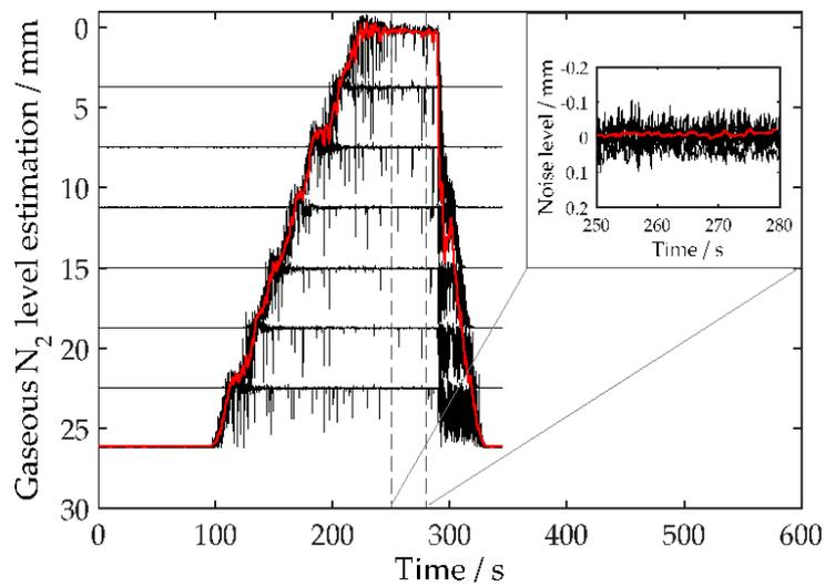
**Figure 4.** Gas level from the transmission measurement in LN<sub>2</sub> (black curve: unfiltered data, red curve: filtered data) during linear emptying and filling procedure of the trap with N<sub>2</sub>.
