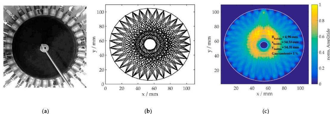
**Figure 6.** Detection of bubble position and size, (a) top-view picture recorded with a camera, (b) reconstructed images from full transmission measurement scans with 224 projections, (c) image post processing (filtering) and circle fitting.
