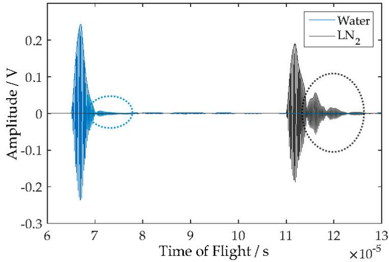
**Figure 3.** Received acoustic signals from a single transmission path measurement in water at 293 K (blue curve) and LN<sub>2</sub> at 77 K (black curve).
