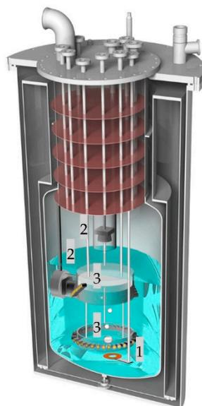
**Figure 2.** Cryogenic measurement setup.
