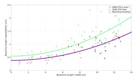
**Figure 2.** Baseline length repeatabilities in CONT17 campaign under different troposphere estimation configuration.
