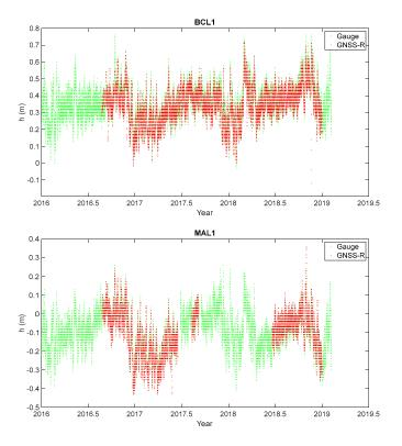
Figure 2. Sea level at BCL1 (up) and MAL1 (down) from GNSS-R IM and tide gauge.
