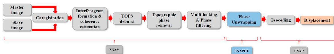
Figure 2. Methodology for the estimation of subsidence in the mining sector.
