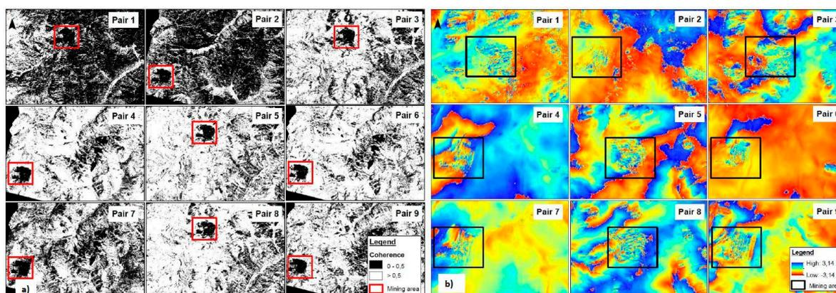
Figure 3. (a) Binary coherence mask; black: coherence < 0.5, white: coherence  $\geq 0.5$ ; (b) Interferograms in the study area.
