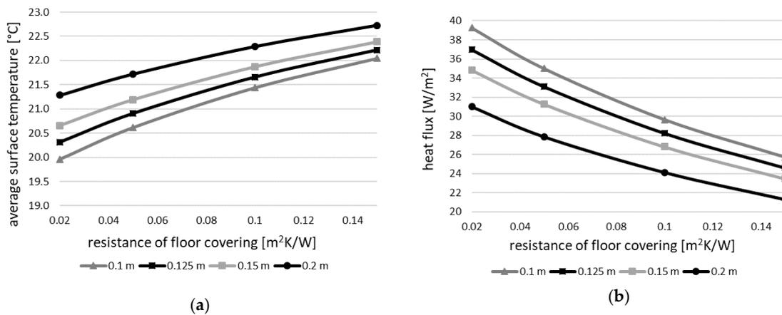
**Figure 3.** Relation between (a) average surface temperature of the cooling floor; (b) heat flux at the surface of the cooling floor, thermal resistance of floor covering for variable pipe spacing (water temperature 16 °C, room temperature 26 °C).
