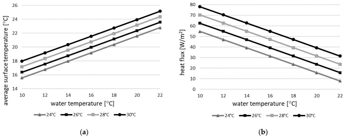
**Figure 2.** Relation between (a) average surface temperature on the cooling floor; (b) heat flux on the surface of the cooling floor, and temperature of the cooling medium for variable room temperature (pipe spacing 0.1 m, thermal resistance of floor covering 0.02 m²K/W).
