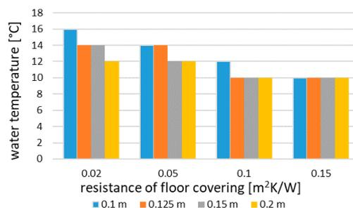
**Figure 4.** Admissible value of water temperature for variable thermal resistance of floor covering and pipe spacing (air temperature 26 °C).
