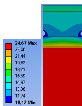
**Figure 1.** Temperature distribution in a floor cooling system (air temperature 26 °C, water temperature 10 °C, resistance of floor covering 0.02 m<sup>2</sup>K/W, pipe spacing 0.1 m).
