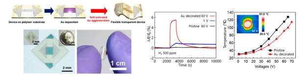
Figure 1. Transparent and flexible Au-decorated graphene microchannel gas sensor (Ref: Kim et al., *Nanoscale*, 2019, 11, 2966–2973).
