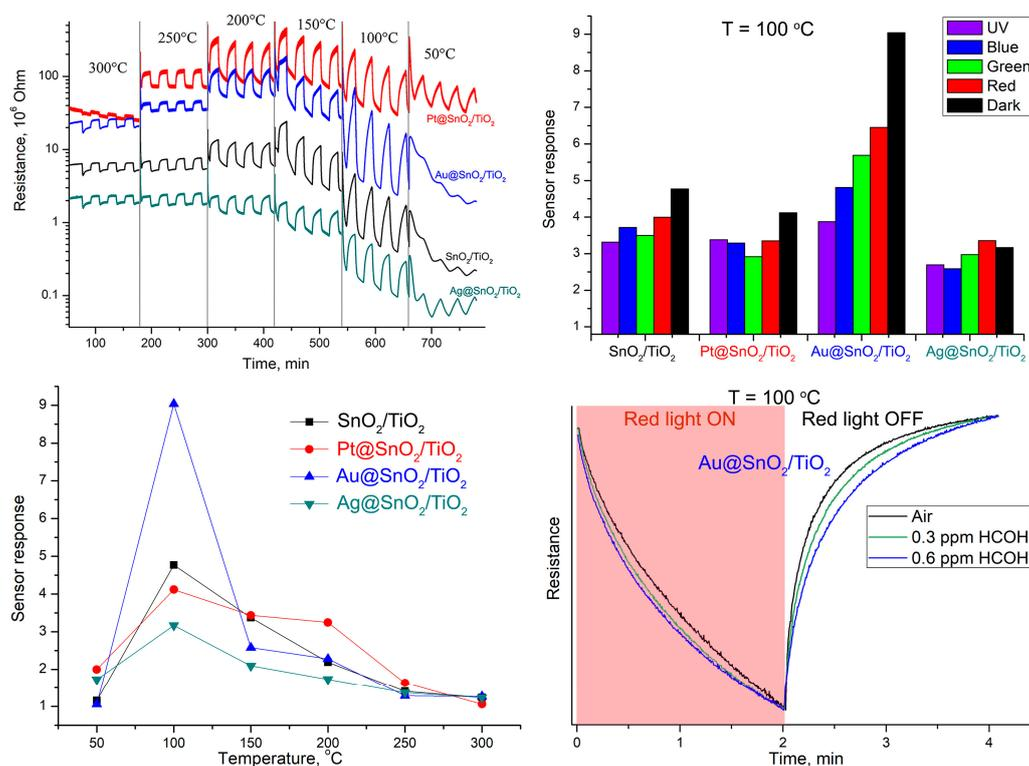
**Figure 1.** (a) Change in the samples resistance at periodic changing the composition of the gas phase; (b) Temperature dependences of sensor response to 0.6 ppm HCHO in dark conditions; (c) Influence of constant illumination on sensor response to 0.6 ppm HCHO at 100 °C; (d) Change in the resistance of Au@SnO<sub>2</sub>/TiO<sub>2</sub> nanocomposites at 100 °C during one “Light ON/OFF” cycle in dry air containing 0, 0.3 or 0.6 ppm HCHO.
