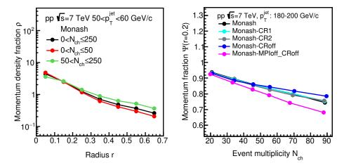
**Figure 1.** (**Left**) The differential jet structure for low and high multiplicites. (**Right**) The integral jet structure at r = 0.2 plotted against  $N_{ch}$  for different MPI and CR simulation settings [5].
