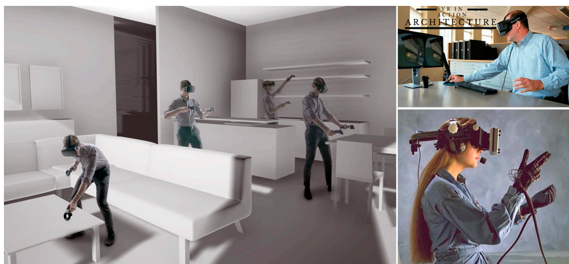
Figure 3. Use of the current advanced Vr technology, including a HMD viewer for pad handling and editing elements, aptic devices and MOCAP tracking gloves.
