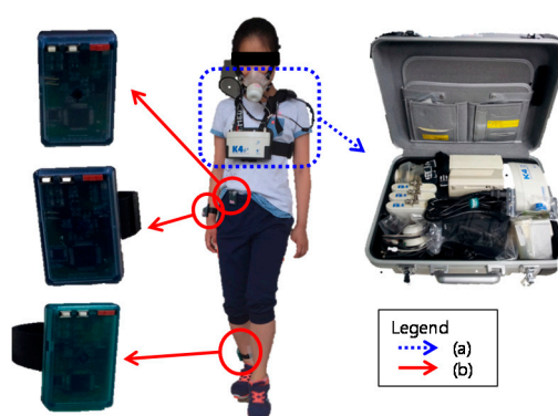
Figure 1. The picture of subject who wears both portable metabolic monitoring device and accelerometer system at the same time. (a) The reference device, portable metabolic analyzer, K4b2. (b) The devised 3-axis accelerometer system which is composed of 3 part module, waist, wrist and ankle.
