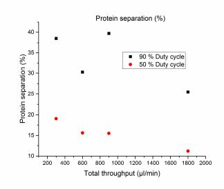
**Figure 4.** Separation test. Protein separation performances depends on the duty cycle of the square wave signal and on the flow rate.
