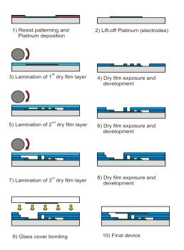
**Figure 2.** Fabrication process. Sequence of steps from the patterning of the electrodes to the glass cover bonding.
