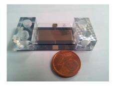
Figure 3. The device equipped with the two acrylic connectors.
