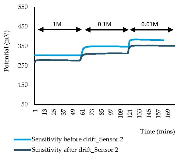
Figure 1. Sensitivity and repeatability tests of Sensor 2.
