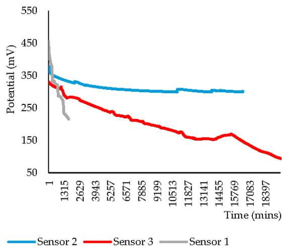
Figure 2. Drift test of Sensors 1, 2, 3 with layer barrier.
