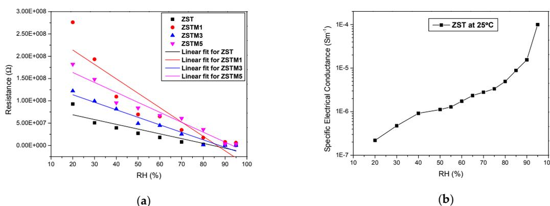
**Figure 2.** (a) Resistance change of the sensors versus relative humidity of 20% to 95% RH at room temperature fitted with the linear lines; (b) humidity dependency of the bulk electrical conductivity for humidity range of 20%–95% RH at room temperature for the ZST micro sensor.
