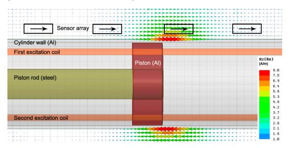
**Figure 3.** Magnetic field component in axial direction outside the pneumatic cylinder simulated by FEM. Excitation field of 4 Hz in radial direction penetrates the aluminum wall and is substantially deformed near the end of the piston rod made of common magnetizable steel. Sensors are oriented in the axial direction and perpendicularly to the excitation field.
