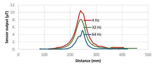
Figure 5. Single sensor output vs. piston position for excitation frequency of 4 Hz, 32 Hz and 64 Hz.
