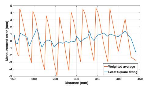
Figure 6. Positioning error throughout the central 300 mm stroke of the pneumatic actuator.
