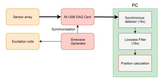
Figure 4. Schematic diagram of signal processing.
