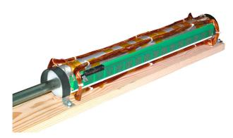
**Figure 2.** The actual position sensor is made of 16 integrated fluxgate sensors and is attached to the pneumatic actuator model which is 50 cm long and 6 cm in diameter.
