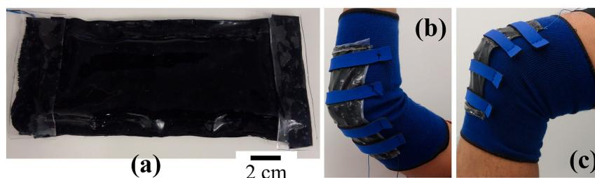
**Figure 2.** Photograph of (a) top view of device; (b) TrEG mounted on elbow; and (c) on knee.
