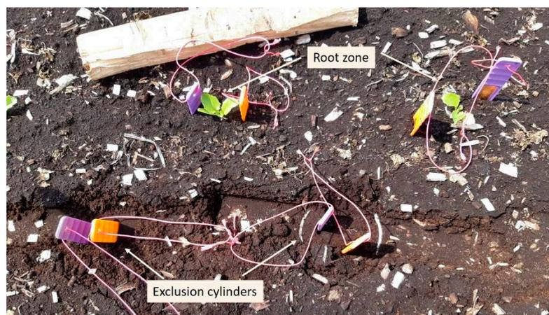
**Figure 2.** Experimental design with PRS<sup>®</sup> probes installed in the root zone and in root exclusion cylinders. The probes are shown here before they were completely inserted into the soil.
