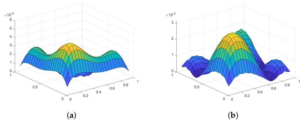
**Figure 6.** Graphical representation of absolute errors for the CN-FDM and the EDGM in Example 1 at  $h = 1/24$ ,  $N = 100$  and  $\gamma(x, y, t) = \frac{1 - (xyt)^3 + \sin(xyt)^2}{10}$ . (a) CN-FDM; (b) EDGM.
