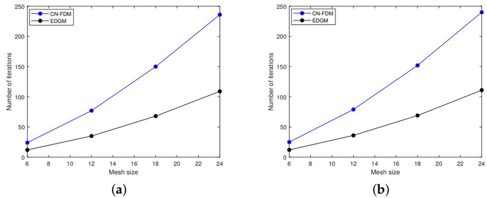
**Figure 8.** Graphical comparison of iterations number for the CN-FDM and the EDGM in Example 2. (a)  $(x, y, t) = \frac{10 - (xyt)^3}{80}$ ; (b)  $\gamma(x, y, t) = 5xt^{-3}$ .
