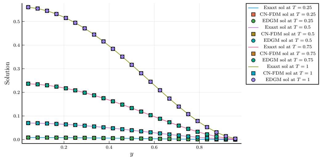
**Figure 5.** Graphical comparison of the exact solution and numerical solutions obtained using the CN-FDM and the EDGM in Example 1 at  $h = 1/24$ ,  $\tau = 0.01$ ,  $y = 0.5$  and  $\gamma(x, y, t) = \frac{16 - e^{xyt}}{17}$ .
