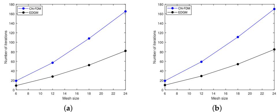
**Figure 4.** Graphical comparison of iterations number for the CN-FDM and the EDGM in Example 1.
