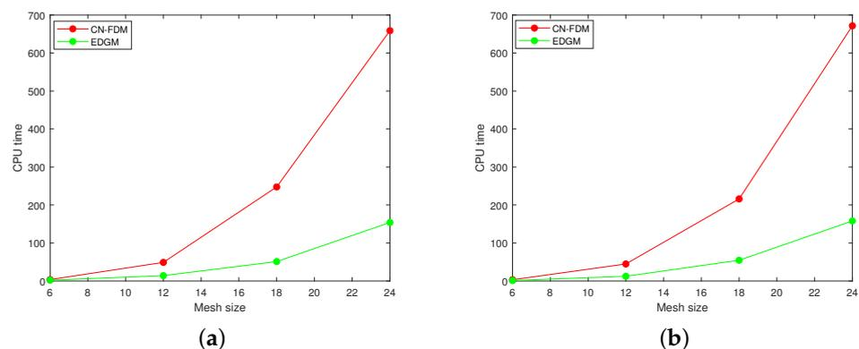
**Figure 7.** Graphical comparison of CPU time for the CN-FDM and the EDGM in Example 2. (a)  $\gamma(x, y, t) = \frac{10 - (xyt)^3}{80}$ ; (b)  $\gamma(x, y, t) = 5^{xt-3}$ .
