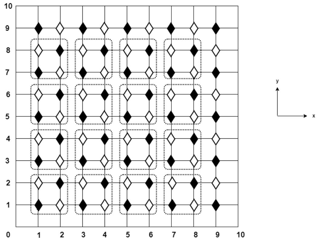
Figure 2. Computational molecule of the EDGM with  $M_x = M_y = 10$ .
