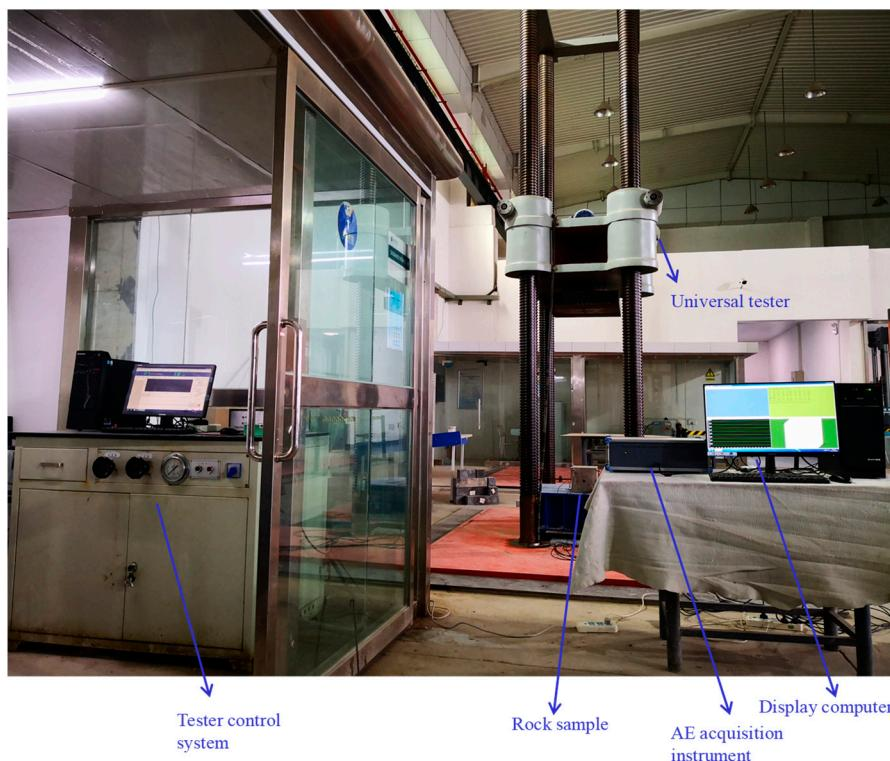
**Figure 1.** General layout of the experimental device.
