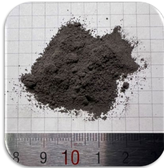
Figure 2. Morphology of regenerated micro-powder.
