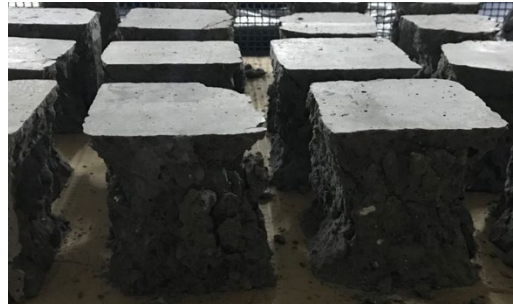
Figure 5. Pictures of compressive strength tests.
