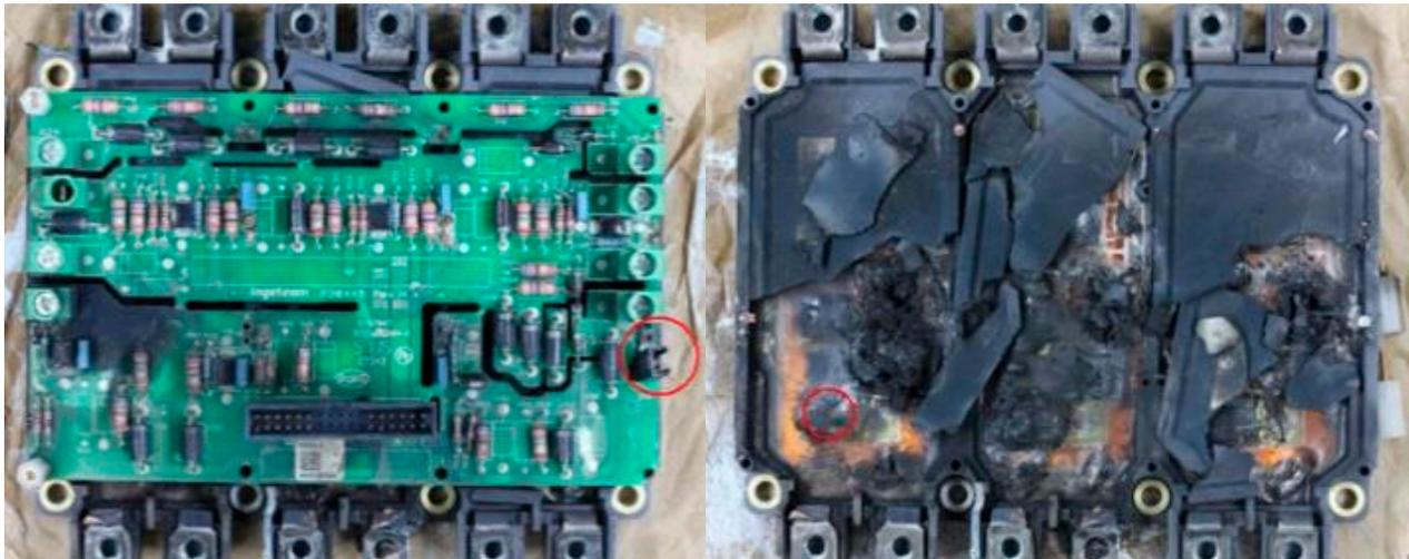
**Figure 2.** (left): IGBT module before failure; (right): IGBT module after failure.
