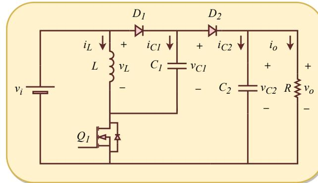
**Figure 1.** Elementary circuit of Super-lift Luo converter.
