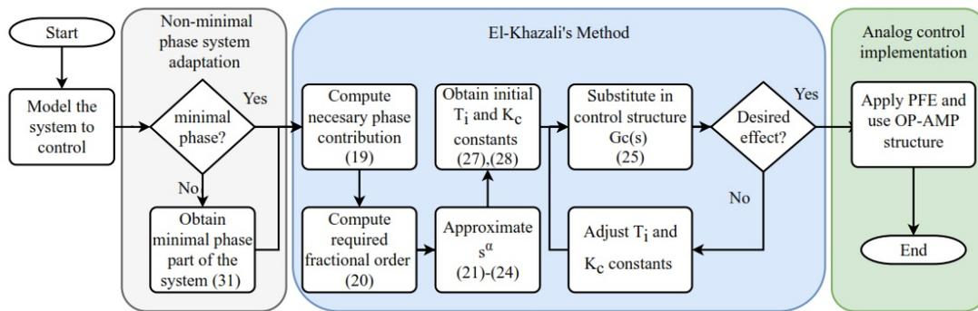
Figure 5. FOC design methodology. PFE = Partial Fraction Expansion.
