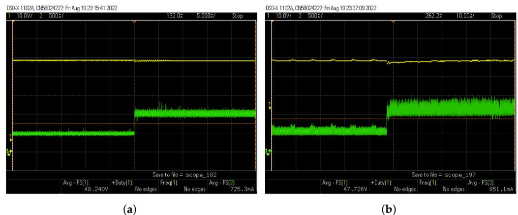
Figure 15. Load variation response, from 50 to 100% load, for the Super-lift Luo converter. (a) FOPID controller, (b) 'I' controller.
