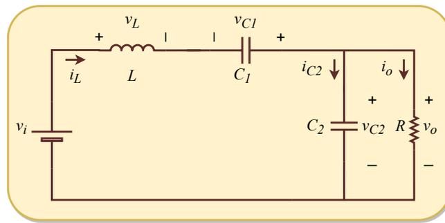
**Figure 3.** Super-lift Luo converter  $t_{off}$  interval.
