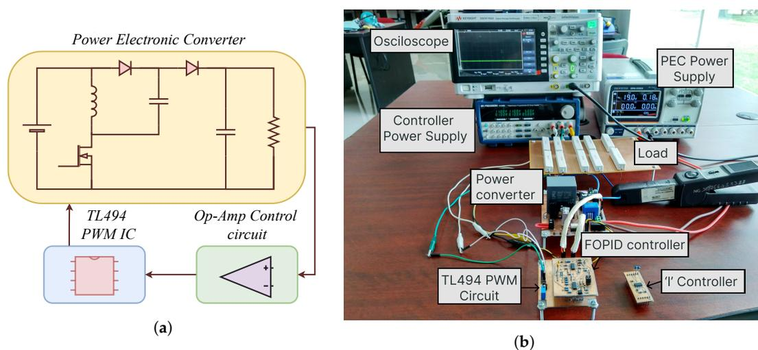
**Figure 13.** Test setup for the Super-Lift Luo converter. (a) Practical set-up block diagram, (b) Practical set-up.
