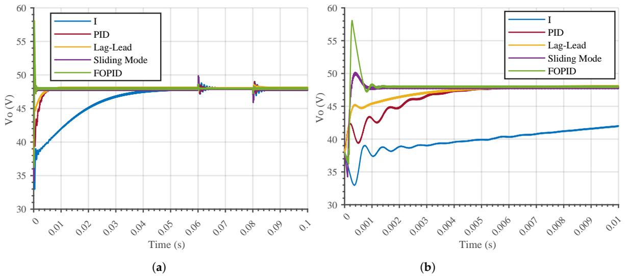
**Figure 11.** PSIM simulation of the Super-lift Luo converter. (a) Complete simulation results, (b) close up on step response.
