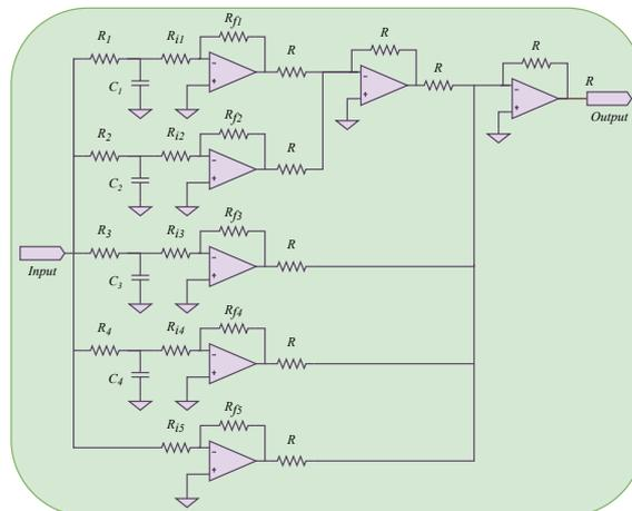
Figure 6. FOPID controller implementation circuit.
