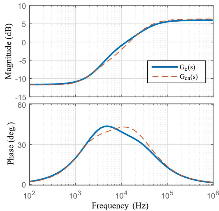
Figure 9. Bode plot of FOPID approximation.
