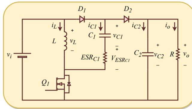
Figure 4. Super-lift Luo converter with one parasitic element.
