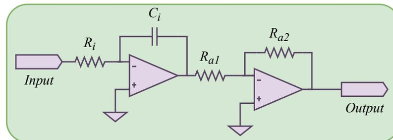
Figure 7. ‘I’ controller implementation circuit.
