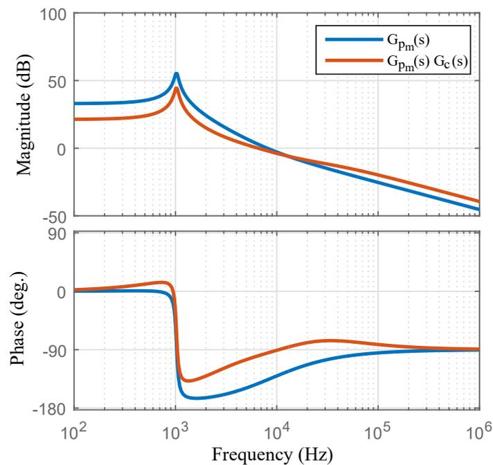
**Figure 10.** Open loop Bode plot of the minimal phase part of the system.
