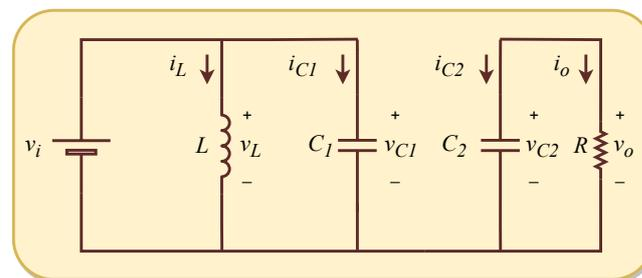
**Figure 2.** Super-lift Luo converter  $t_{on}$  interval.
