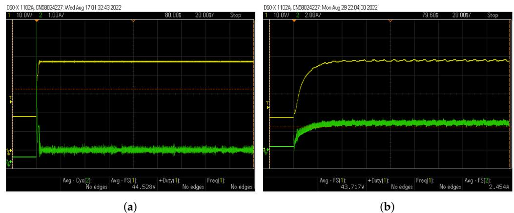
Figure 14. Step response for the Super-Lift Luo converter. (a) FOPID controller, (b) 'I' controller.
