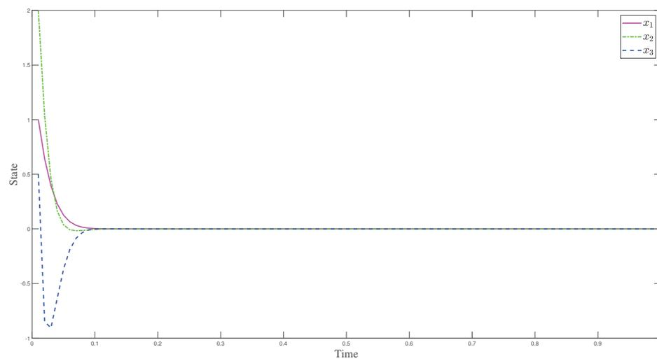
Figure 2. States of system (14) with respect to time under controller (15) with  $T = 0.01$ .
