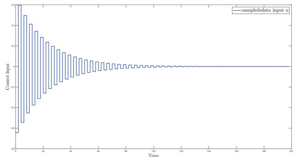
**Figure 9.** Sampled-data input of system (14) in function of time under controller (16) and  $T = 2$ .
