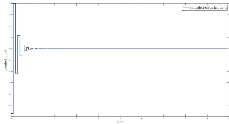
**Figure 6.** Sampled–data input of system (14) in function of the time under controller (15) and  $T = 0.1$ .
