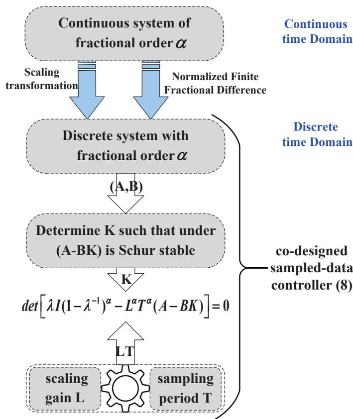
Figure 1. Procedure of identifying the parameters in the co-designed sampled-data controller (8).
