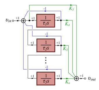
Figure 2. FLF block diagram for implementing LP, HP, BP, BS and AP filter functions.
