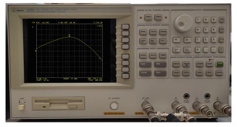
**Figure 6.** Screenshot of the Agilent 4395A spectrum analyzer, showing the gain frequency response during the measurement of the BP type of filter for orders ( $\alpha$ ,  $\beta$ ) = (0.7, 0.4).
