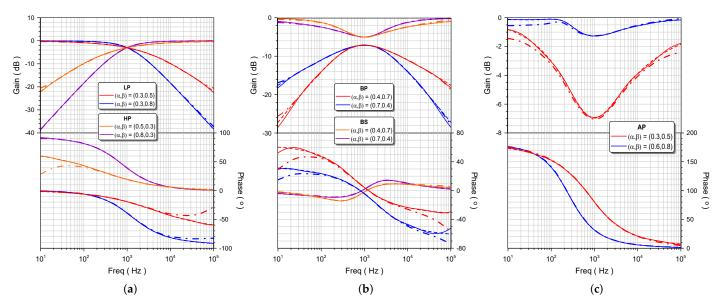
**Figure 1.** Gain and phase frequency responses, derived from 5th-order Oustaloup (dashed-dotted lines) and 5th-order curve-fitting-based (solid lines) approximation methods, for the (**a**) LP and HP, (**b**) BP and BS and (**c**) AP filter cases given in Table 2, along with the corresponding ideal responses (dashed lines).
