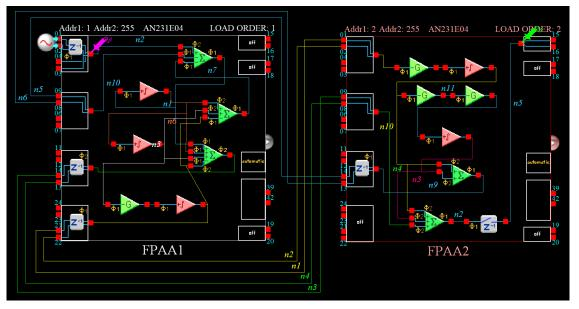
Figure 3. FPAA-based realization of the functional block diagram in Figure 2.
