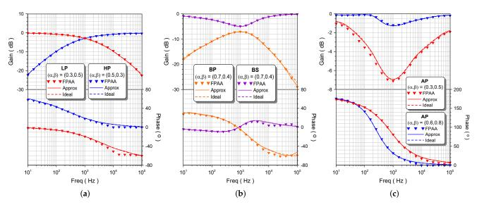
**Figure 5.** Experimental gain and phase frequency responses (triangle symbols), along with the corresponding approximated (solid lines) and ideal (dashed lines) responses, for (**a**) LP and HP, (**b**) BP and BS and (**c**) AP filter cases.
