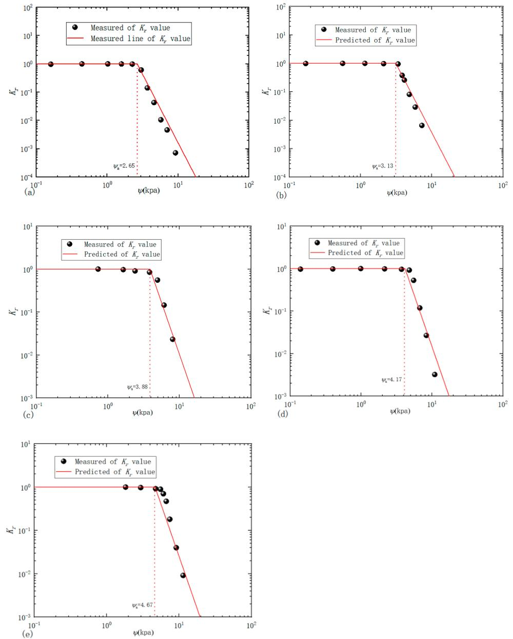
**Figure 5.** Prediction results of the unsaturated relative permeability coefficients of Columbia sandy loam with different void ratios: (a)  $e = 1.268$ ; (b)  $e = 1.114$ ; (c)  $e = 0.942$ ; (d)  $e = 0.89$ ; (e)  $e = 0.815$ .
