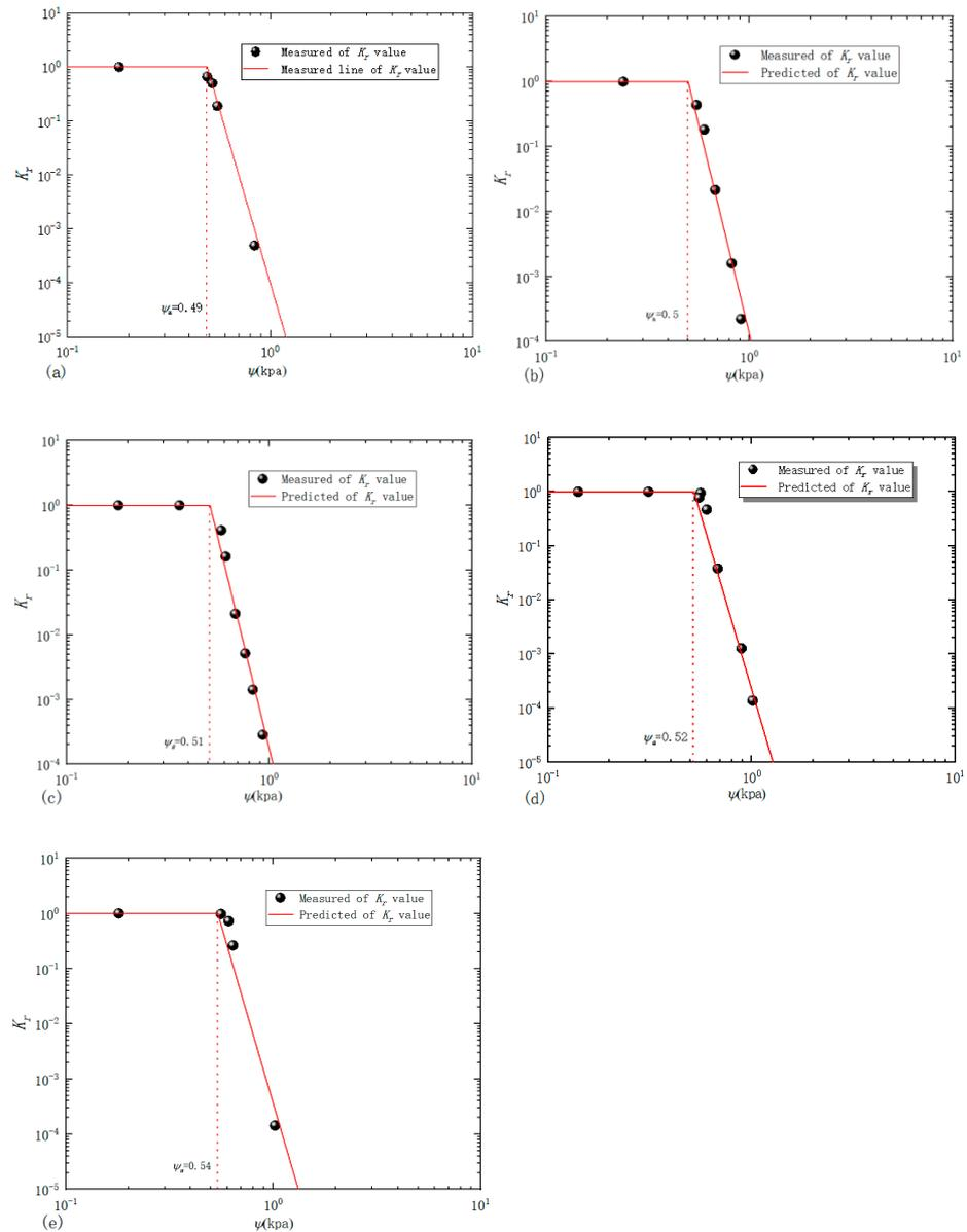
**Figure 6.** The prediction results of the unsaturated relative permeability coefficients of unconsolidated sand with different porosity ratios: (a)  $e = 0.852$ ; (b)  $e = 0.825$ ; (c)  $e = 0.799$ ; (d)  $e = 0.767$ ; (e)  $e = 0.715$ .
