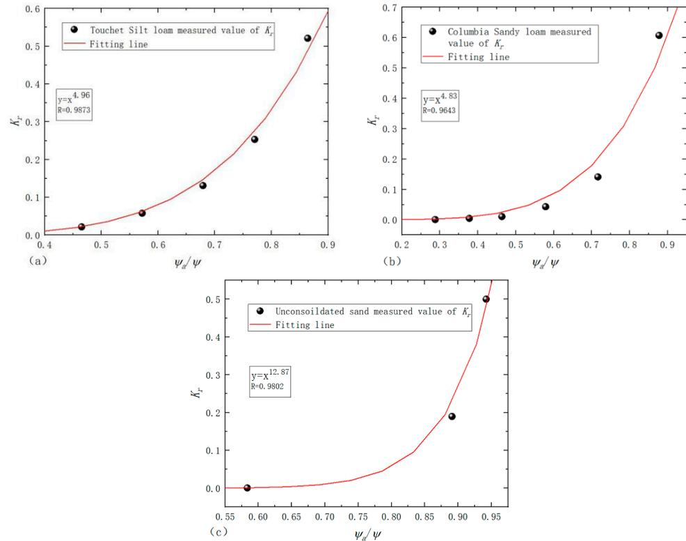
**Figure 3.** Fitting values of  $\lambda$  for three types of soil: (a) Touchet silt loam; (b) Columbia sandy loam; (c) unconsolidated sand.
