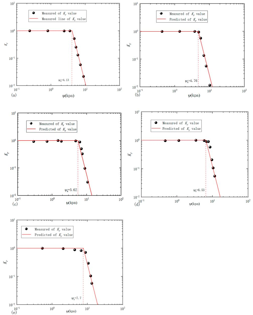
**Figure 4.** Touchet silt loam's different porosity ratio unsaturated relative permeability coefficient prediction results: (a)  $e = 1.012$ ; (b)  $e = 0.916$ ; (c)  $e = 0.815$ ; (d)  $e = 0.733$ ; (e)  $e = 0.653$ .
