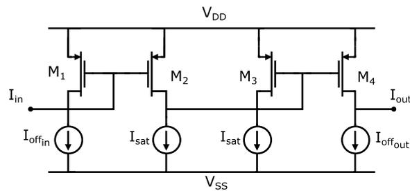
Figure 14. CMOS design of the SNLF block taken from [36].
