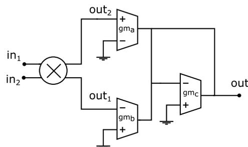
Figure 13. Proposed single-ended multiplier combining the fully-differential multiplier shown in Figure 11 and an OTA-subtractor.
