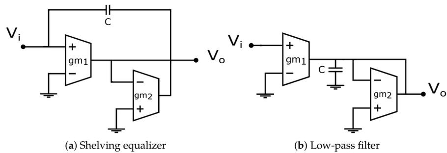
**Figure 4.** OTA-based first-order active filters taken from [33], to implement: (a)  $H_1(s)$  and  $H_2(s)$ , and (b)  $H_3(s)$ .
