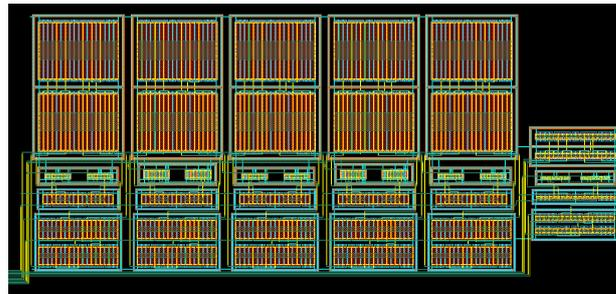
**Figure 16.** Layout of our proposed OTA fractional-order integrator to approximate  $1/s^{0.9}$ .
