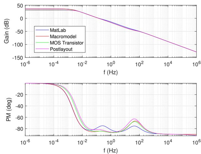
**Figure 17.** Comparison of the gain (up side) and phase margin (down side) responses of the fractional-order integrator  $H(s) = 1/s^{0.9}$ , considering the ideal transfer function approximation in MATLAB, macro-modeling the OTAs, HSPICE simulation using MOS transistor models, and post-layout simulation.
