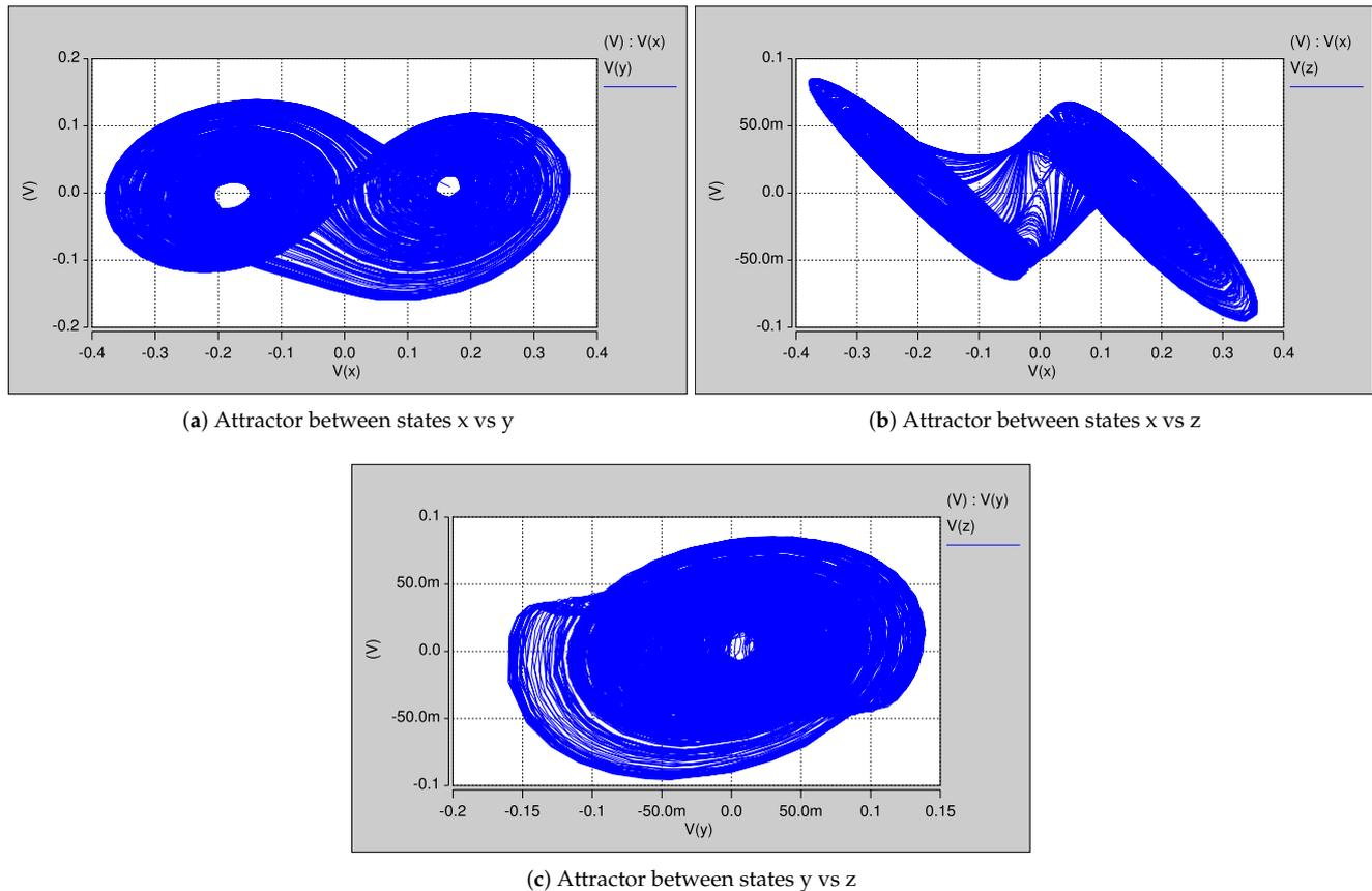
**Figure 9.** Portraits of the HSPICE simulation of FOCO<sub>2</sub> from Figure 8.
