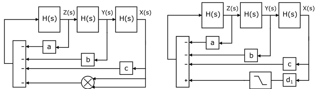
(a) FOCO<sub>1</sub> can be synthesized by three fractional-order integrators, amplifiers, one adder with 4 negative inputs, and one multiplier to evaluate X(s)\*X(s) from (4).
