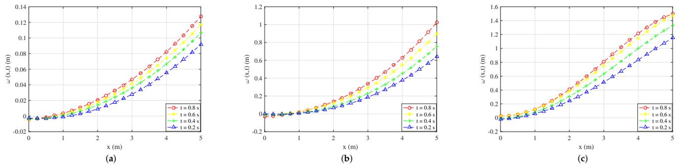
**Figure 3.** Numerical solutions of the displacement of polyurea beam at different moments and different loads: (a)  $f(x, t) = 10$  N, (b)  $f(x, t) = 2x$ , (c)  $f(x, t) = \sin 2t$ .
