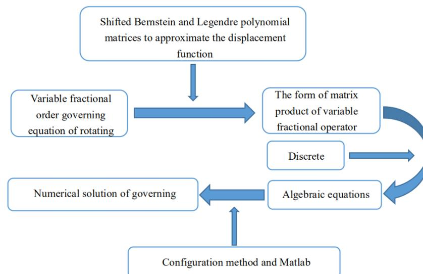
**Figure 2.** Schematic diagram of the shifted Bernstein–Legendre polynomial collocation algorithm.
