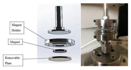
Figure 8. Design of top plate (left) and entire test assembly (right).
