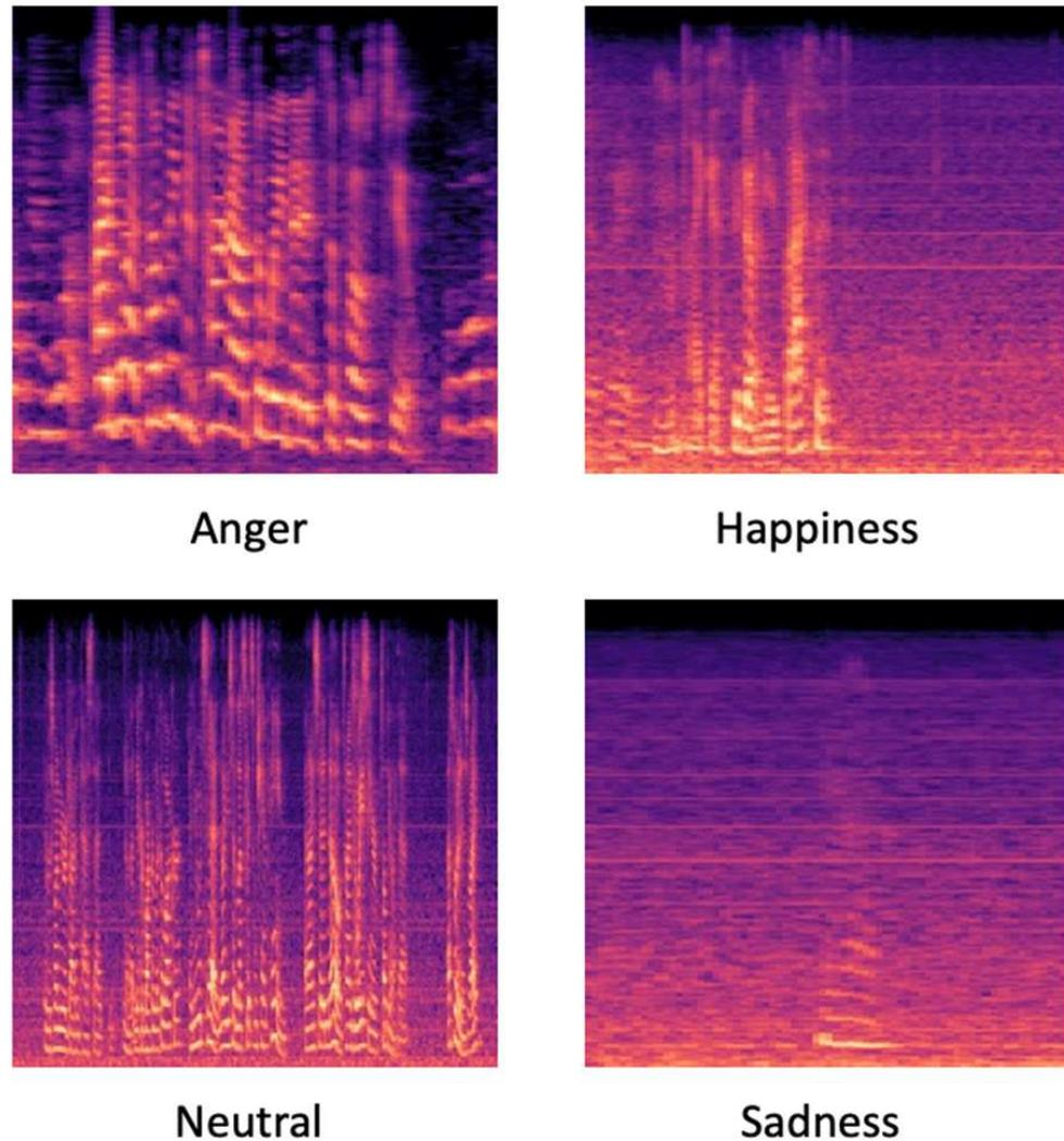
**Figure 3.** Differences between classes Mel spectrogram.
