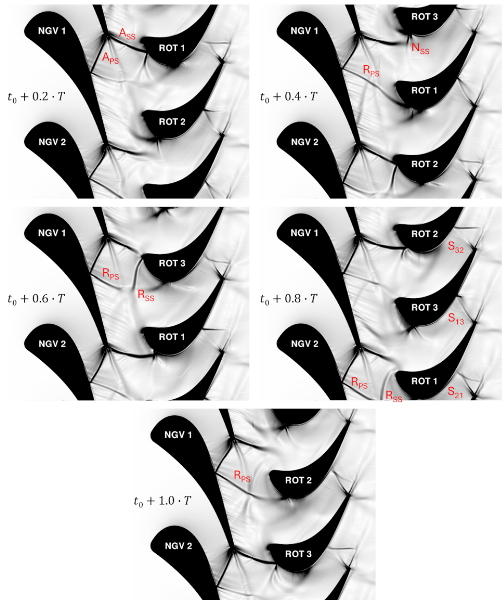
Figure 10. Numerical Schlieren visualization of the shock system occurring in the CT3 high-pressure turbine stage at mid-span (adapted from [123]).
