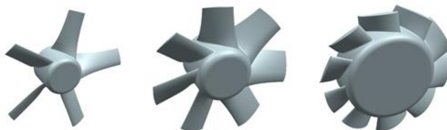
Figure 1. Typical axial impellers with increasing hub-to-tip ratio from left to right (classic blade shape); duct-type casing is not shown.
