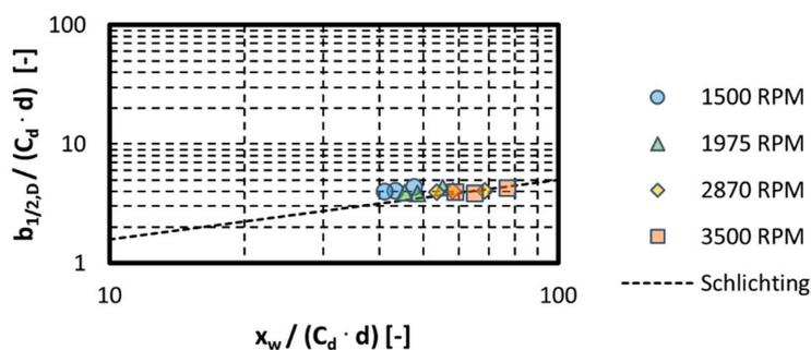
Figure 8. Wake half-width  $b_{1/2,D}$  with respect to wake propagation length  $x_w$ .
