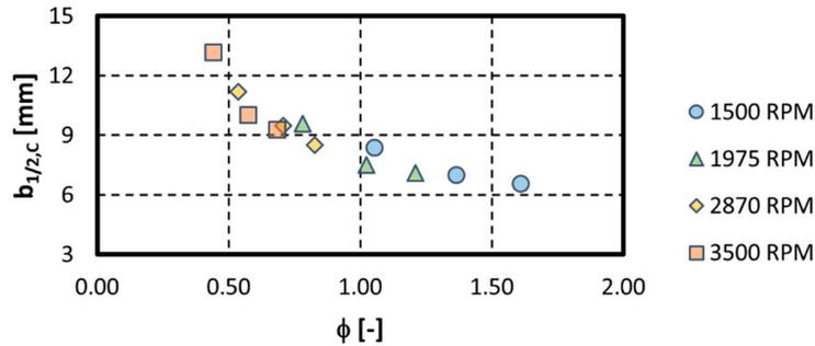
Figure 7. Wake half-width  $b_{1/2,C}$  with respect to flow coefficient  $\phi$ .
