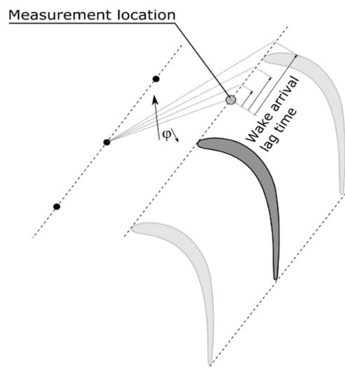
Figure 6. Influence of flow coefficient  $\phi$  on wake propagation length  $x_w$  and on wake arrival lag time.
