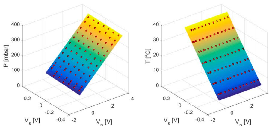
**Figure 1.** Pressure (left) and temperature (right) calibration surface fits for 5 PSI absolute pressure Kulite sensor; red dots indicate 91 calibration points.
