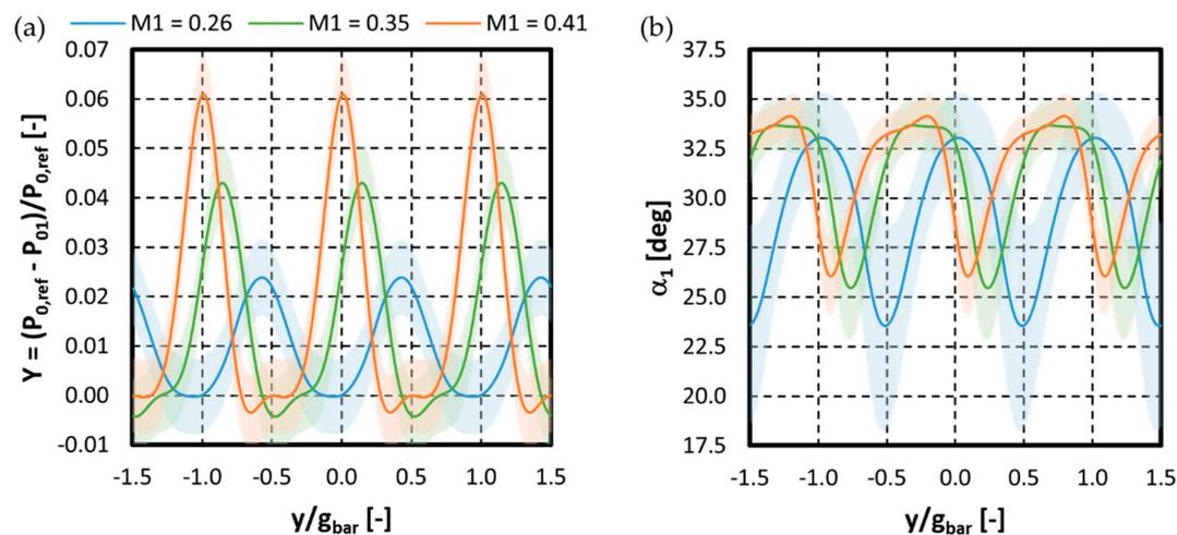
**Figure 4.** (a) Relative total pressure drop in the bar wake; (b) inlet flow angle variation in the bar wake;  $\Omega_{rot} = 2870$  RPM at  $M_{1,is} = 0.26$  (blue),  $0.34$  (green) and  $0.41$  (orange) for 96 bars.
