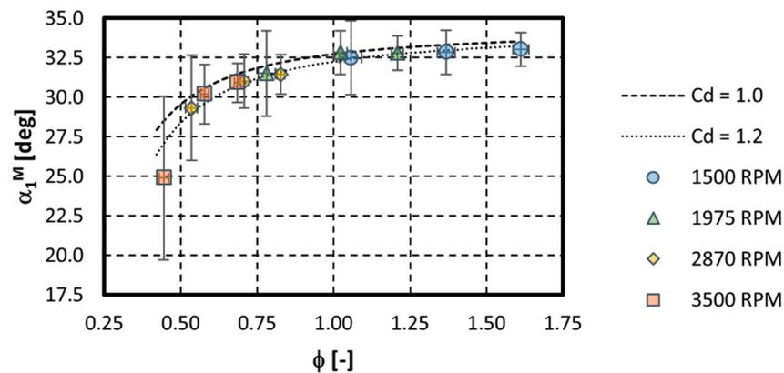
**Figure 11.** Evolution of the mass-averaged absolute inlet flow angle with respect to the flow coefficient; theoretical results are plotted for two cylinder drag coefficients:  $C_d = 1.0$  and  $C_d = 1.2$ .
