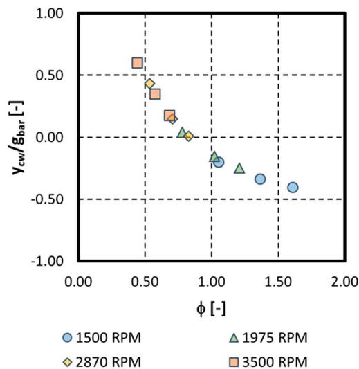
Figure 5. Normalized wake center location with respect to flow coefficient  $\phi$ .
