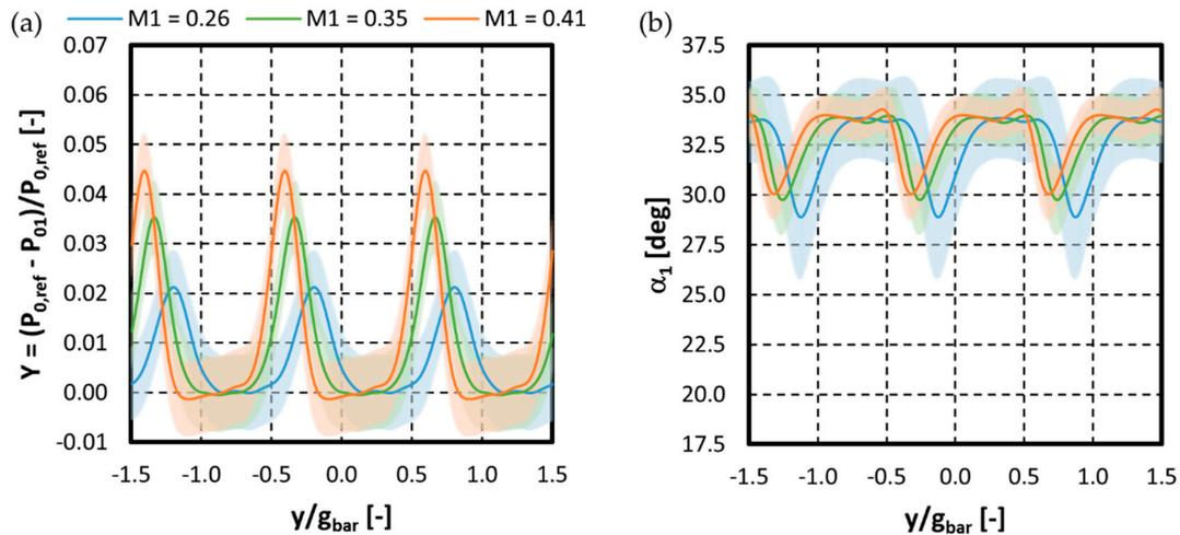
**Figure 3.** (a) Relative total pressure drop in the bar wake; (b) inlet flow angle variation in the bar wake;  $\Omega_{rot} = 1500$  RPM at  $M_{1,is} = 0.26$  (blue),  $0.34$  (green) and  $0.41$  (orange) for 96 bars.
