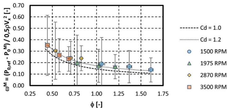
**Figure 10.** Evolution of the mass-averaged total pressure loss coefficient with respect to the flow coefficient; theoretical results are plotted for two cylinder drag coefficients:  $C_d = 1.0$  and  $C_d = 1.2$ .
