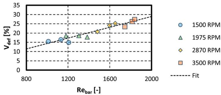
**Figure 9.** Evolution of the velocity deficit ratio in the wake  $V_{def}$  as a function of bar-relative Reynolds number  $Re_{bar}$ .
