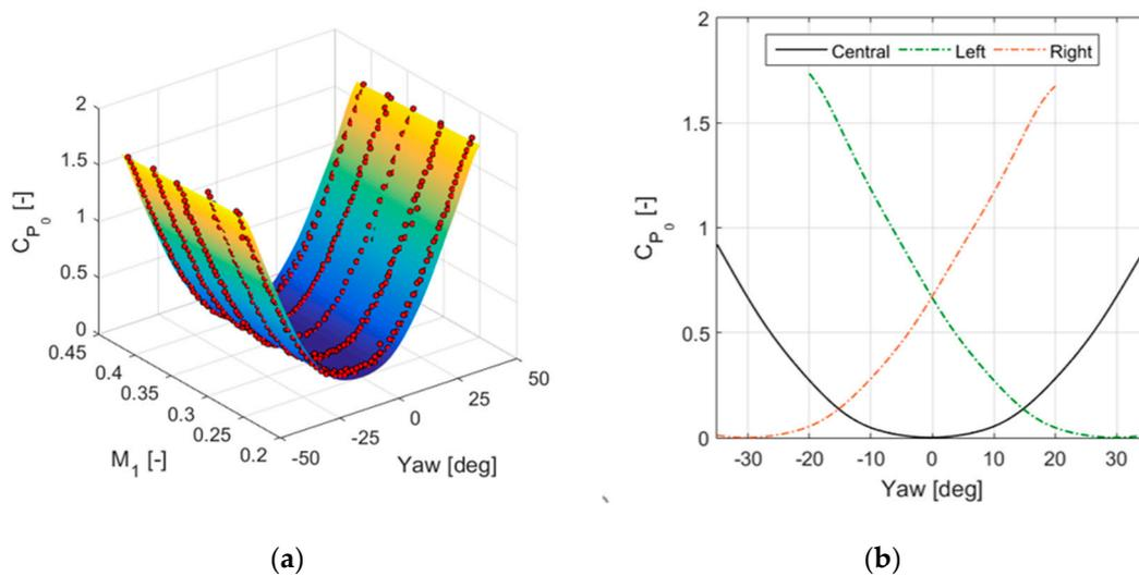
**Figure 2.** (a) Pressure recovery coefficient  $C_{P_0}$  surface fit of a single sensor probe; red dots indicate 505 calibration points; (b) derived angular calibration for the virtual three-hole mode at  $M_1 = 0.42$ .
