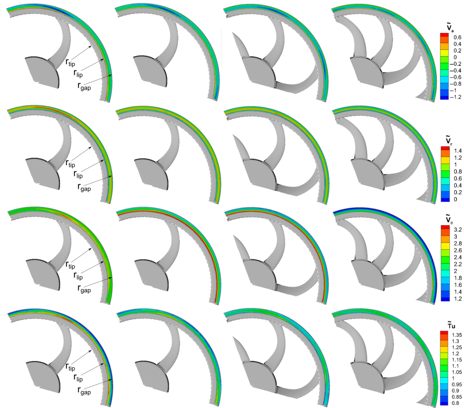
Figure 7. Phase-averaged distributions of velocity components and turbulence intensity level acquired by means of LDV instrumentation within the gap at x/r_{tip} = -0.0225 .
