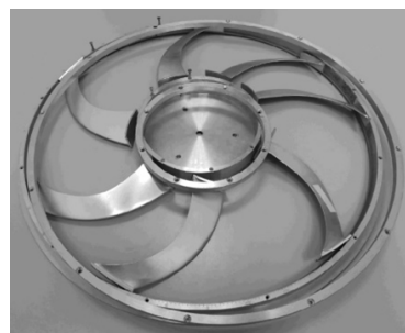
Figure 2. Unmounted aluminum variable geometry rotor.
