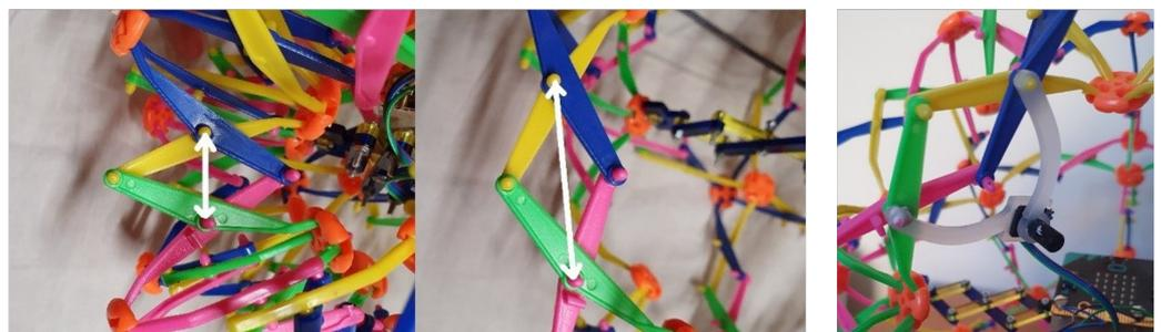
**Figure 3.** (Left) Change in angle of SLE when open versus closed; (Right) potentiometer mounted as an auxiliary SLE.
