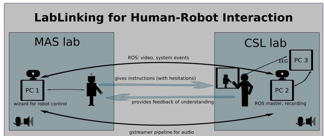
**Figure 1.** The LabLinking setup for conducting HRI studies between the laboratory of the Medical Assistance System Group (MAS) at Bielefeld University and the Cognitive Systems Lab (CSL) at the University of Bremen: The Pepper robot gives instructions to the human interaction partner, which provides feedback of understanding. The laboratories are connected via a GStreamer pipeline for audio and additional communication via ROS for video and further system events.
