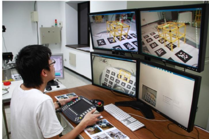
**Figure 5.** The 4-monitor setup for presenting the video feed from four camera views [7] (used with permission from Elsevier). The recommended lifting path (the yellow dotted line) is overlaid into the video feed to help operators avoid collisions.
