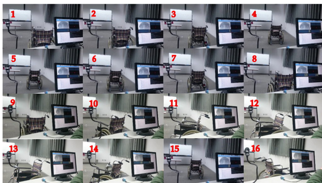
Figure 21. Eye blink control wheelchair travel experiment.
