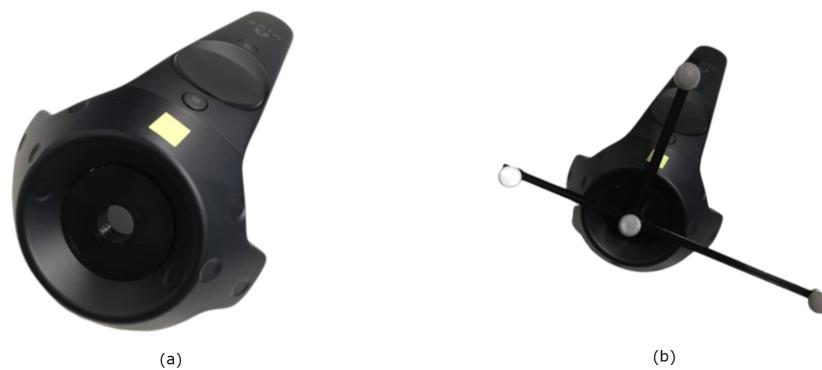
**Figure 6.** HTC Vive controller: (a) Calibration setup. (b) Tracking setup.
