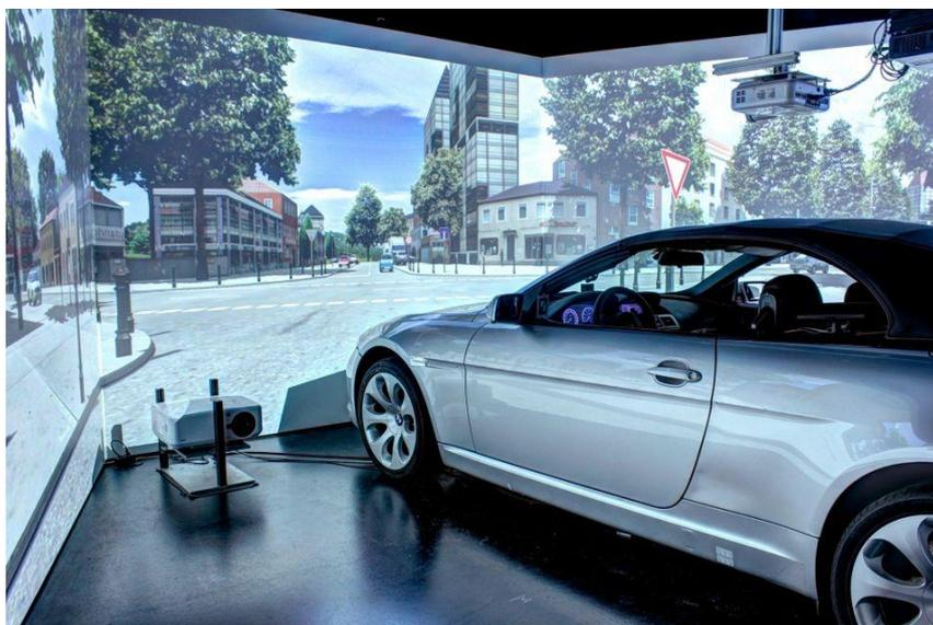
**Figure 1.** Driving simulator used for the study.
