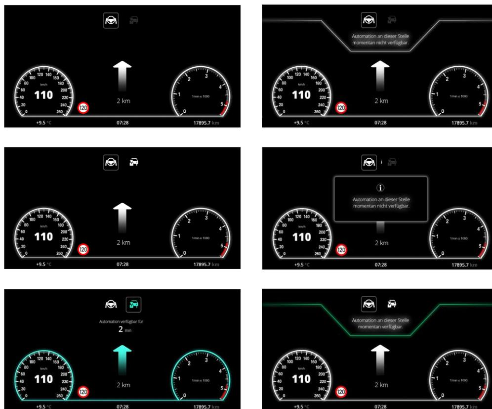
**Figure 3.** Human–machine interface (HMI) concepts: **(Top left):** Manual driving; **(middle left):** Automation available; **(bottom left):** Automation activated; **(top right):** Context-adaptive non-availability notification; **(middle right):** Pop-up with non-availability notification; **(bottom right):** Context-adaptive availability notification.
