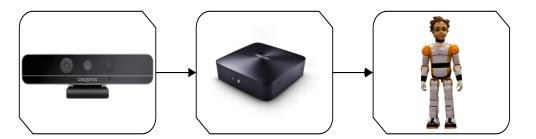
**Figure 1.** Experimental setup. Starting from the left: Intel<sup>®</sup> RealSense<sup>™</sup> (model F200), computer and ZECA robot.
