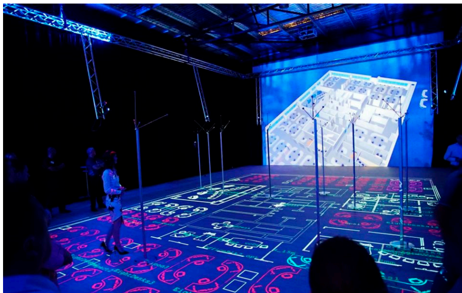
Figure 1. CADwalk installation showing projected building blueprints and rendered view on rear wall (head-mounted-display (HMD) view not shown).
