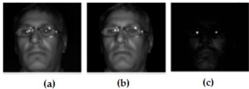
Figure 1. How to obtain driver pupils from two images. (a) bright-eye image; (b) dark-eye image; (c) difference image [21].
