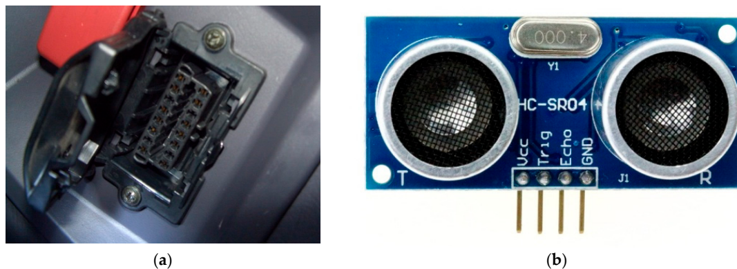
Figure 3. Vehicle driving sensors. (a) On-board diagnostics connector [34] (b) Ultrasound sensor for outside obstacle detection [35].
