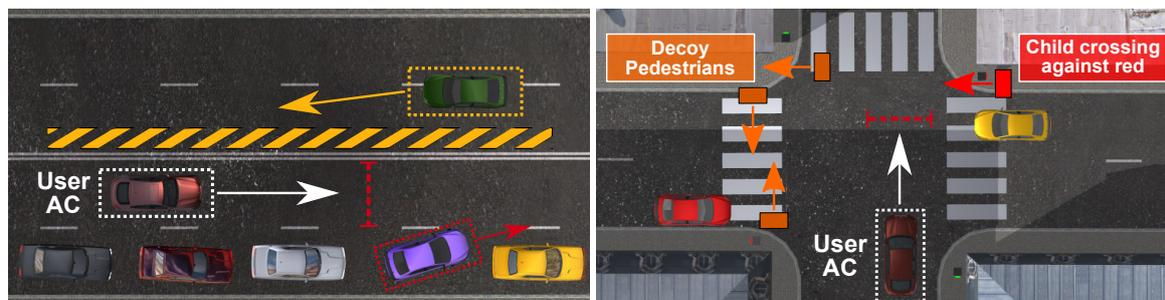
**Figure 3.** Top-down view on exemplary driving situations from Table 2. (Left) a *standing traffic hazard* with one car pulling out late from a parking spot in front of the approaching AC, forcing it into full braking; (Right) an *imminent head-on collision* case with a child emerging from cover to cross the road. Decoys provide additional stimuli for a more realistic scene, best viewed in color.
