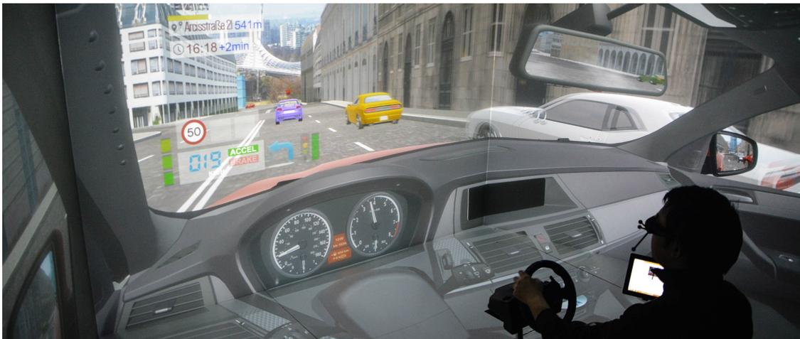
**Figure 4.** The basic study setup of our driving simulation in the MR environment. The driver is seated in front of the (ineffective) steering wheel. Rendered in 2D for better visibility, best viewed in color.
