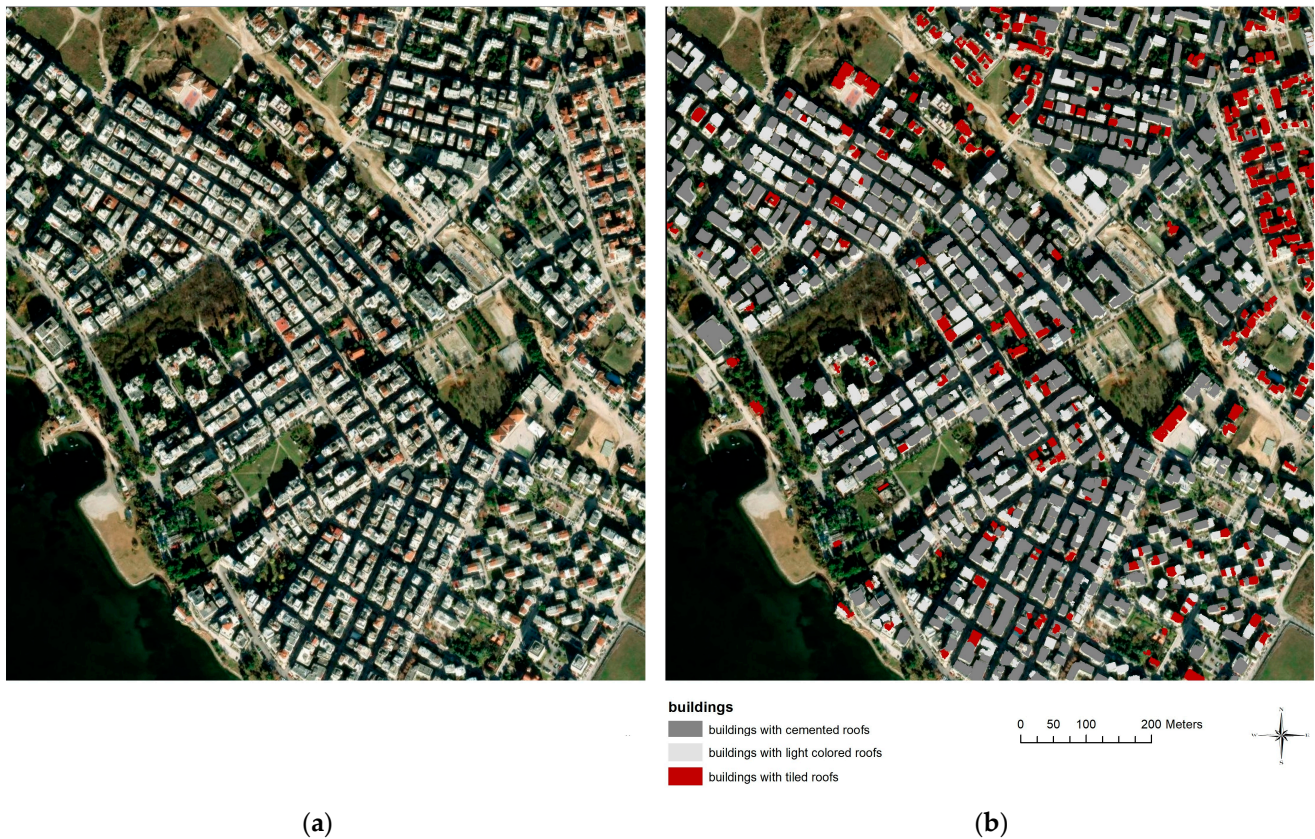
Figure 3. Classification of buildings with the RF classifier: (a) the WorldView-2 image, (b) the buildings classified by their roof types; (1) buildings with tiled roofs, (2) buildings with cement roofs, (3) buildings with light-colored roofs.
