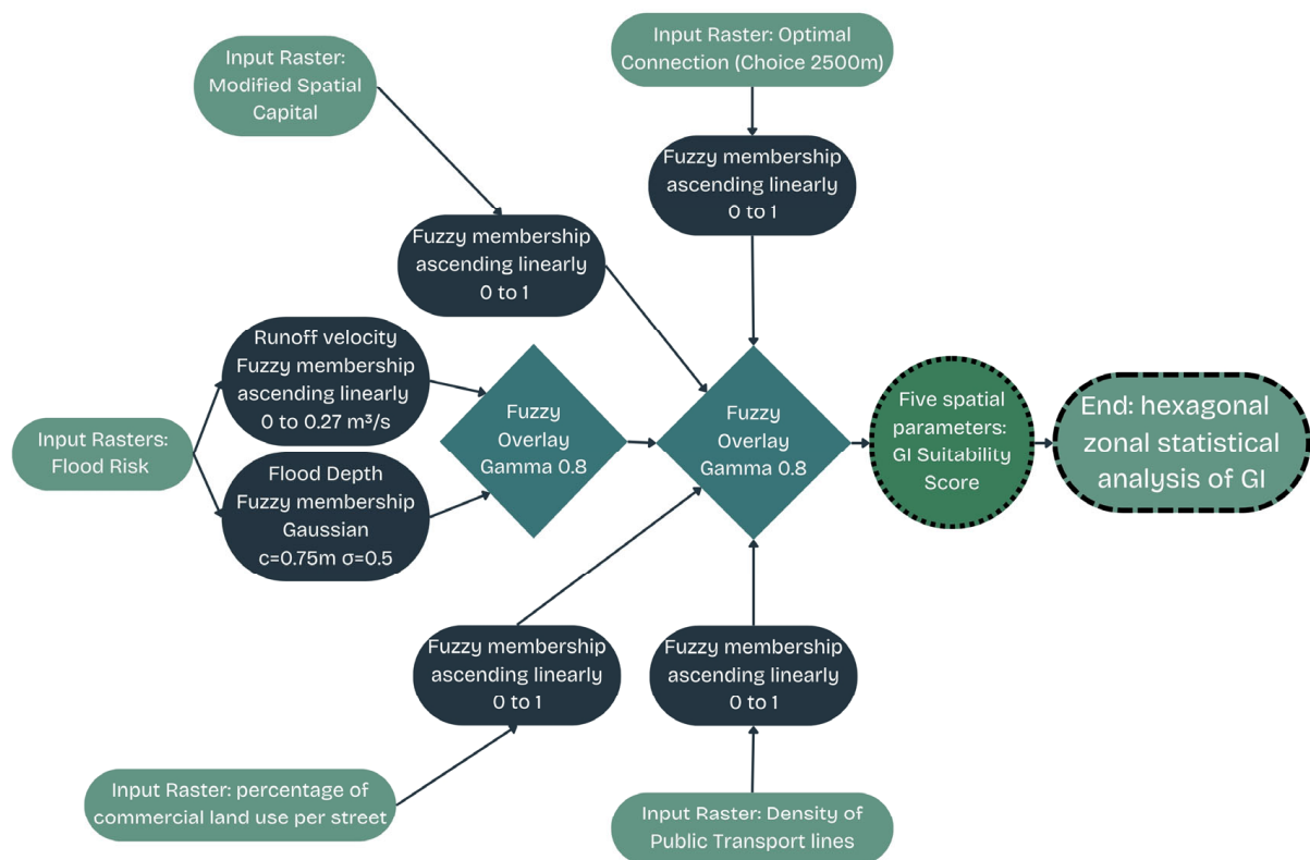
Figure 6. Fuzzy logic diagram stating grouped inputs, membership functions, overlay stages, and the final suitability output.
