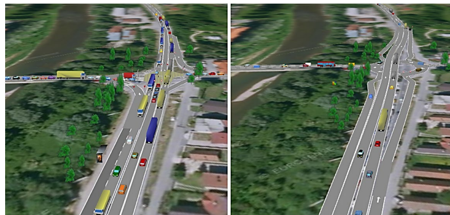
Figure 9. The multi-level intersection proposal via Aimsun software.
