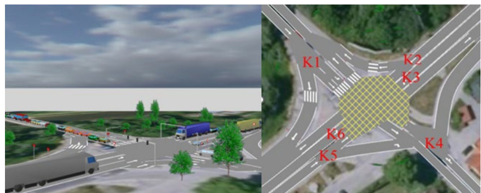
Figure 4. Creating queues at the intersection during the simulation and marking directions.
