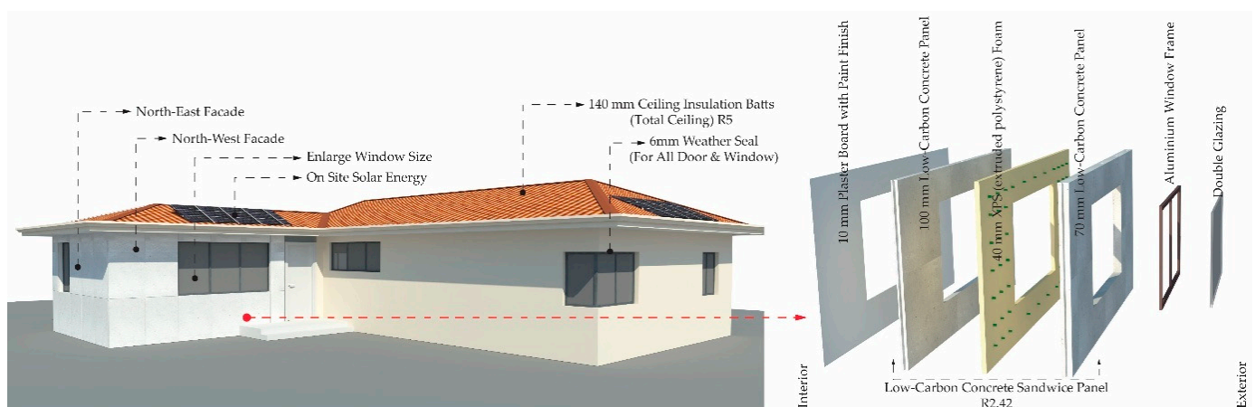
Figure 13. The views show Case Study 2 after retrofitting and prefabricated plugin installation details.
