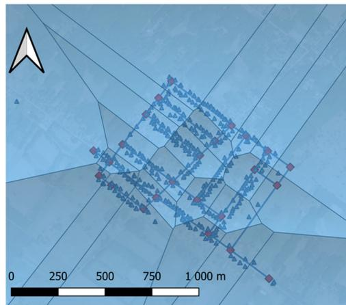
**Figure 10.** Determination of the nodes' range of influence based on Thiessen polygons. Red squares are the connection nodes, blue triangles are the consumption points.
