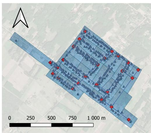
**Figure 9.** Manual determination of the nodes' range of influence. Red squares are the connection nodes, blue triangles are the consumption points.
