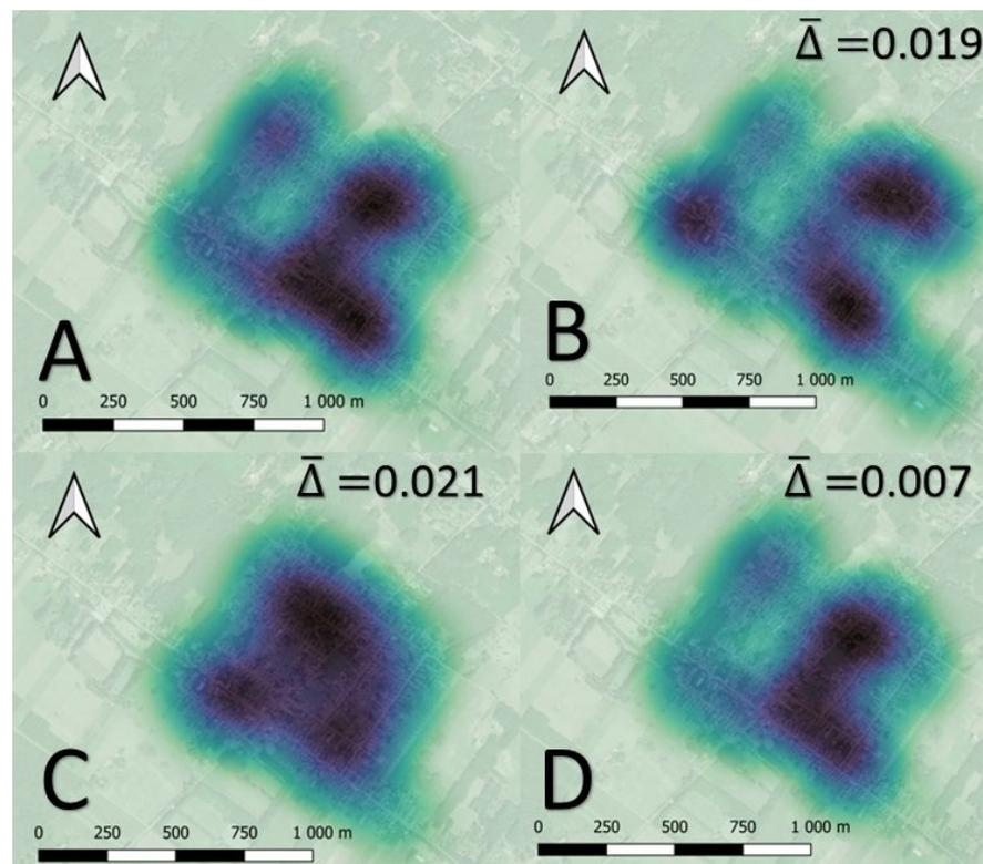
**Figure 11.** Consumption heat maps based on manual method (A), zoning based on the street (B), arithmetic average (C), and Thiessen polygons (D).
